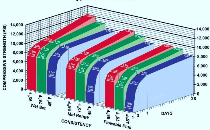
A cement-based, non-shrink, premixed, highly flowable grout that develops extremely high compressive strengths in a very short period of time.
