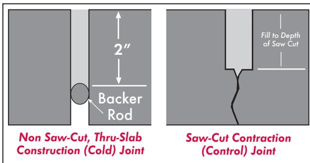
In construction (formed) joints that are not saw-cut, **Edge-Pro 80** should be installed at a minimum 2" depth. **DO NOT USE COMPRESSIBLE BACKER ROD IN STANDARD SAW-CUT CONTRACTION/CONTROL JOINTS!** Rod may be used 2" down in construction or saw-cut joints exceeding 2" in depth ONLY.
