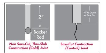
In construction (formed) joints that are not saw-cut, **Edge-Pro 80** should be installed at a minimum 2" depth. **DO NOT USE COMPRESSIBLE BACKER ROD IN STANDARD SAW-CUT CONTRACTION/CONTROL JOINTS!** Rod may be used 2" down in construction or saw-cut joints exceeding 2" in depth ONLY. Moderate-Duty Semi-Rigid Polyurea Joint Filler for Retail and Warehouse Concrete Floors
