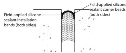
**Fig.3: BEJS System in Existing Steel Angles – Retrofit**
