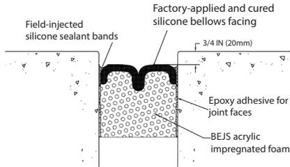
**Fig.2: BEJS-ON-A-REEL for Joints 1/2" (12mm) – 1 1/4" (30mm)**
